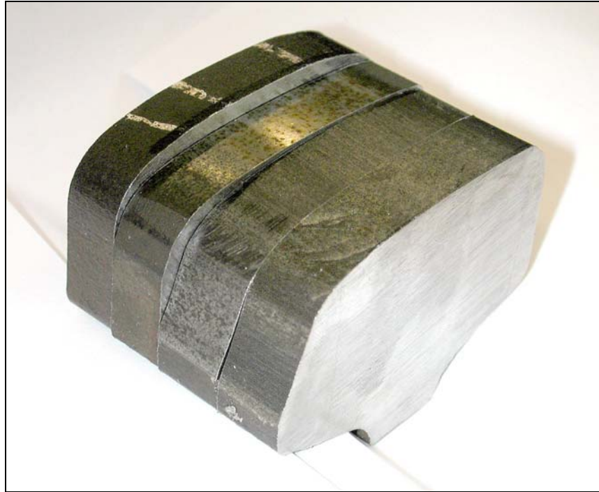
Figure 1. Transverse slices from rail samples A-B-C-D showing degree of wear.
