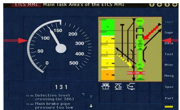
Prospective early development DMI interface for ERTMS equipped UK HST power units
