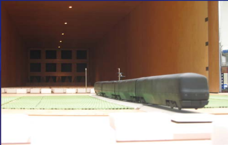
Class 365 EMU 30 th scale model. Forces measured at several yaw angles
