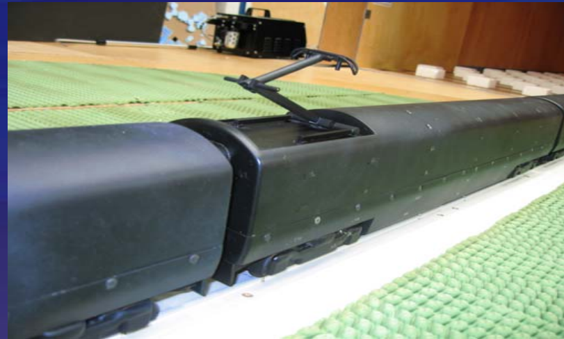
Class 365 EMU 30 th scale model. Forces measured at several yaw angles
